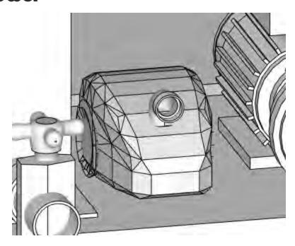
The Blower (seen above in the centre of the drawing) provides additional air flow which increases the force of the jets as the air and water mixes inside the Gunite bodies. The air lines are on top of the Gunite bodies. The blower's shape may change from above but the power will be +/- 900W. There are two 1" to 1.5" bushes that will be needed to connect the blower to the non-return valve and then the 1" pipe to the jets.
