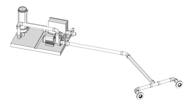
The diagram shows how the drains need to be connected to the pump. The drawing above is expanded so you can clearly see what parts connect to which pipes. Actual placement may change on site. There are additional 90 degree 2" connections in the bill of materials to allow the position to change if needed.
