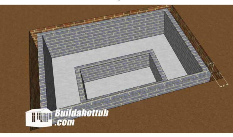
Firstly, you need to remember that there will be plumbing and the minimum size for the Gunite Body fixtures would be 6" (150mm) cavity. You would then be able to fit insulation around the pipes and have a rebar structure inside of the cavity which you would then fill with concrete for the final stage. The drawing below shows what the construction would look like.
