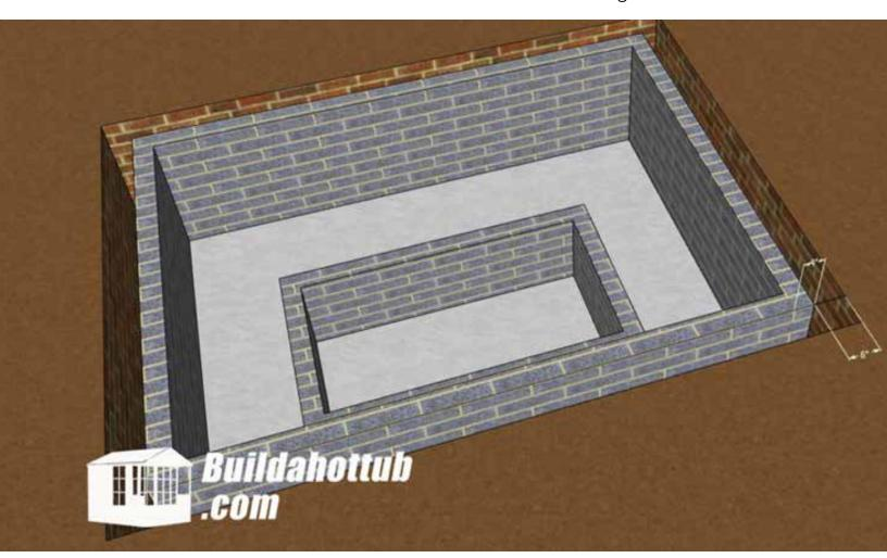
Firstly, you need to remember that there will be plumbing and the minimum size for the fixtures would be 6" (150mm) cavity. You would then be able to fit insulation around the pipes and have a rebar structure inside of the cavity which you would then fill with
