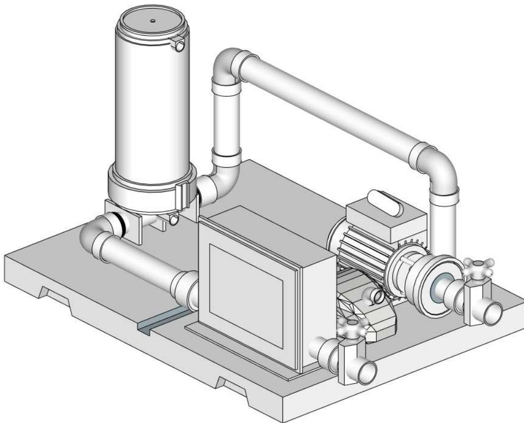
There is a non-return valve placed onto the blower to ensure water cannot pass into the blower. The shape of the blower may vary from the drawing above but the functionality is the same.
